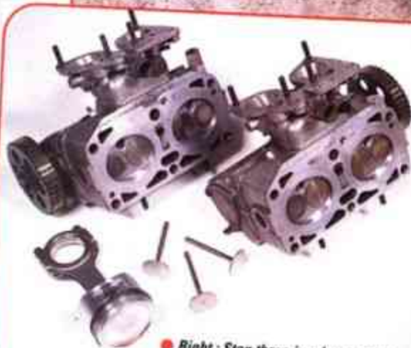
Right: Step three involves a new BLS head which incorporates larger valves
