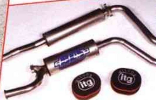
● Above: A pair of filters and a two inch exhaust system net you an extra 10bhp according to BLS
