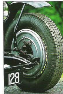
Above: Front suspension on the 6C 2300 was very simple, and followed the standard design of the age with a solid beam axle and semi-elliptic leaf springs controlled by friction dampers. One area, however, where the Alfa scored over the opposition was in its brakes; the enormous finned drums took up most of the space within the wheel rim and provided excellent stopping power. This was almost as much of an advantage on the racetrack as the twin-cam's power.
