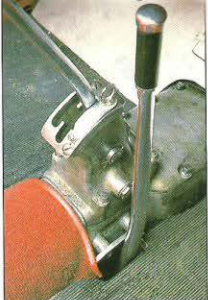
Above: The Alfa had a four-speed manual gear change. As in later Ferraris, the gear lever moved through a metal gate. The handbrake operated on all four wheels via levers and rods.
