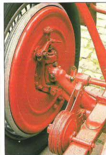
Above: Front suspension on the 6C 2300 was very simple, and followed the standard design of the age with a solid beam axle and semi-elliptic leaf springs controlled by friction dampers. One area, however, where the Alfa scored over the opposition was in its brakes; the enormous finned drums took up most of the space within the wheel rim and provided excellent stopping power. This was almost as much of an advantage on the racetrack as the twin-cam's power.
