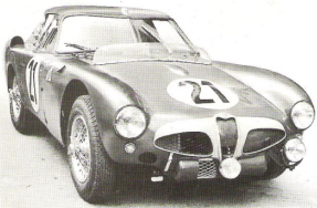
For 1953 the car lost its ovaloid shape and gained a crude but handsome coupé body and a 3.5-litre, 260hp engine
