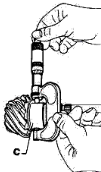
Inspecting interference fit.
