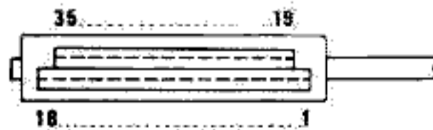
View of multiple conductor connector from system wiring. Terminal 1 (coil) connected to rev. counter.
